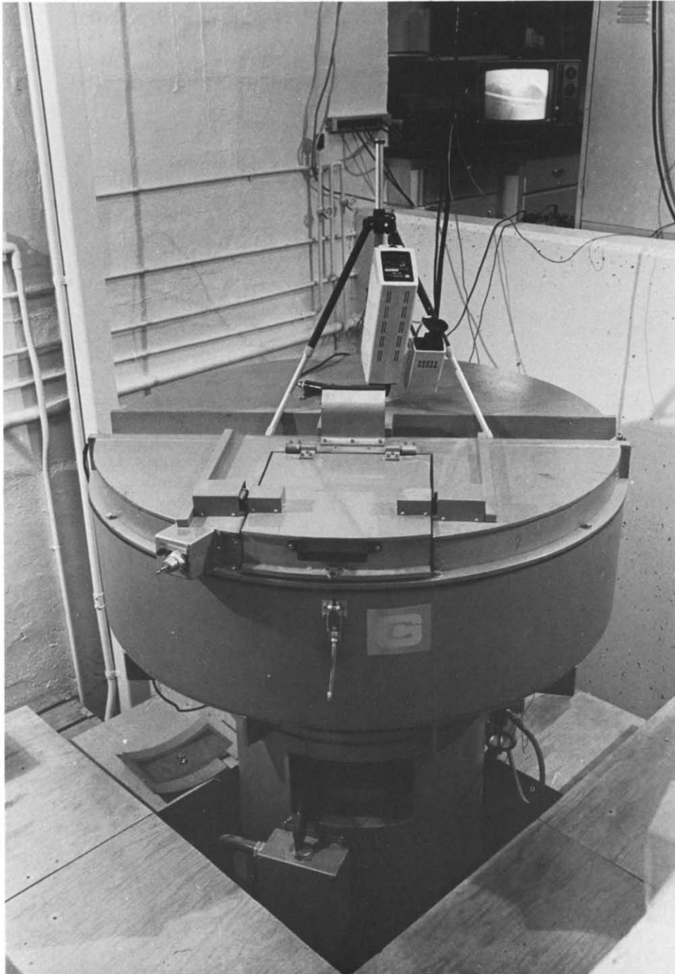
Fig. 1. General view of the 20,000 g centrifuge at Queen's University. Note view of model chamber on TV screen (top right).
